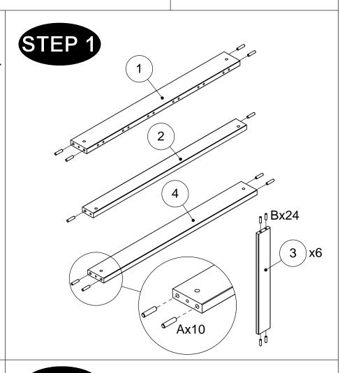
Attach headboard-bottom rail "1", headboard-top rail "2" and headboard-vertical rails "3" together.
