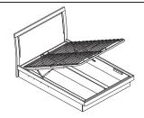
1) Two people carefully lower the slat frame onto the piston bracket . Secure by threading bolts (J) to slat frame on the piston bracket .
