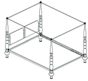
Loosen the metal balls on top of posts, align the top section of the posts in right angle. And insert the canopy rails (7)(8) into holes on top posts (4).
