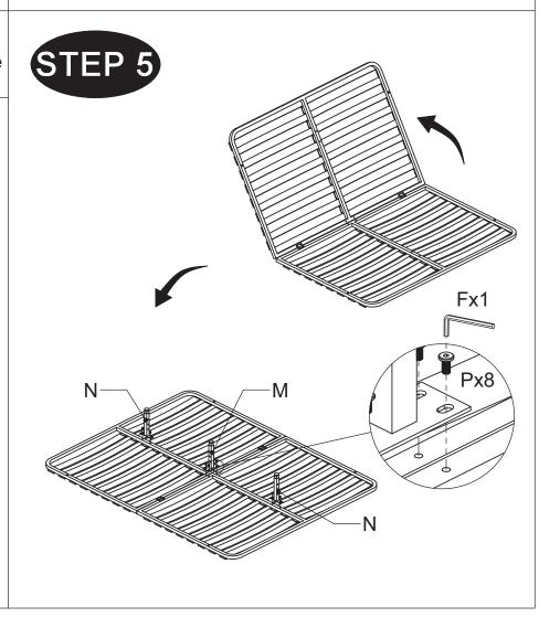
Turn the metal slat frame falling upward and carefully lower the slat frame into the bed.
