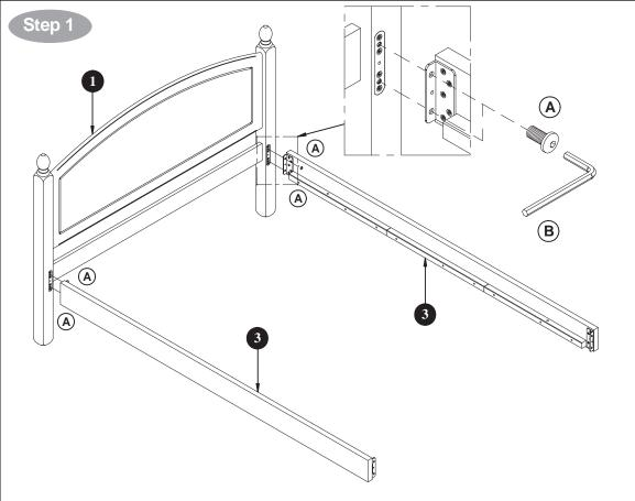
Fix the footboard "2" to the siderail "3" using bolts "A" as shown.
