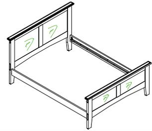
1) Screw the connecting bolt (B) into the headboard (1) and footboard (2).
