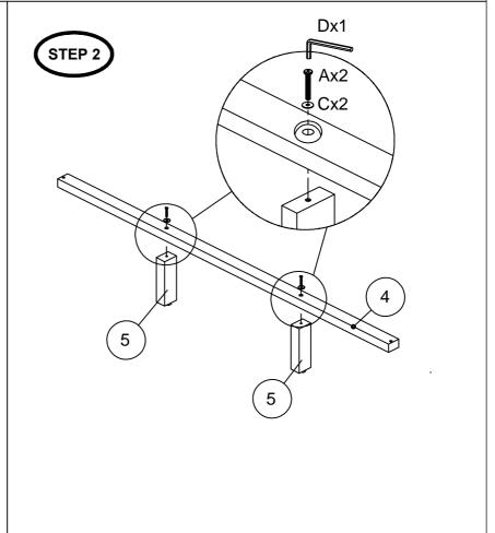
Place the fixed central support "4" onto the support block on headboard "1" and footboard "2".
